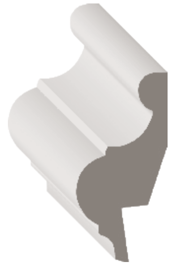
STOCK CODE 6PM (1522168) DIMENSIONS 1 1 / 16 " x 2" x 8-16' ADJUSTABLE 1/4" X 3/4" RABBET PIN
